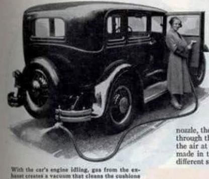
USING the exhaust gas of the automobile to clean the upholstery is the accomplishment of a recently invented device. An aluminum attachment is fastened to the exhaust pipe and the engine is allowed to idle. As the exhaust gas passes through this device suction is created at the inlet hole. Collected by a
